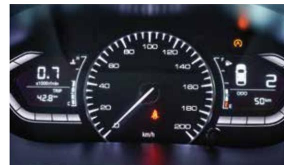
The digital RPM screen provides you with all the vehicle information without letting go of the steering wheel. It indicates fuel consumption pattern, distance to empty, trip meter, gear shift reminder for manual drive and all door open indicator to ensure safety and ease of mind.
